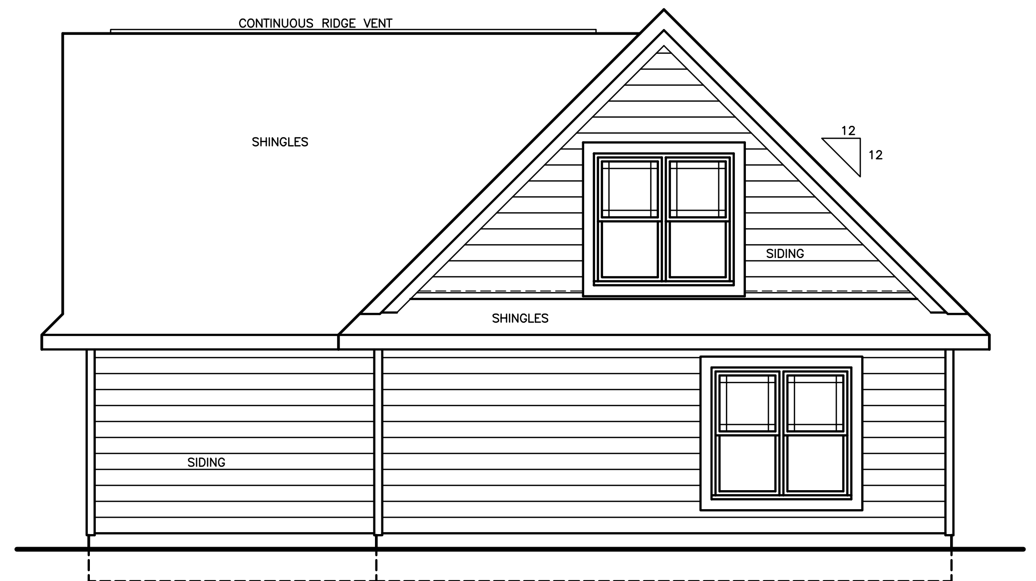
REAR ELEVATION SCALE : 1/4" = 1'-0"
